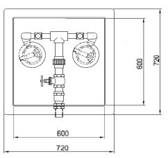
NOTE: no connections to be put through the lid as this inhibits easy removal of the lid for cleaning tank. (Note: tank MUST be positioned in such a way that lid can be removed easily to allow access to tank interior and pump cleaning)
