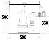
**NOTE:** no connections to be put through the lid as this inhibits easy removal of the lid for cleaning tank. (Note: tank MUST be positioned in such a way that lid can be removed easily to allow access to tank interior and pump cleaning)
